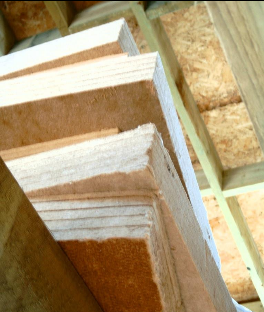
Floor Insulation made from Waste Timber Fibres
