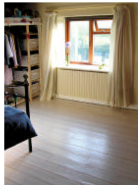
Floor: Osmo Polyx Oil Skirting: Green Paint gloss Walls & radiator: Green Paint satin emulsion
